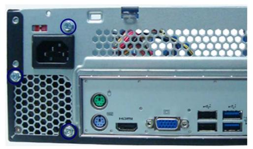
3. Secure the power supply to the chassis using the screw.
